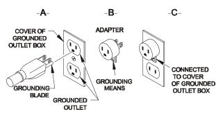
NOTE: The use of the adapter shown in figures B and C is not permitted in Canada.
