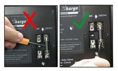
If your charger can accommodate 208 or 230/240 volt input, and has a cover plate, remove the two side screws. If necessary, remove the fuse as shown. Press it into other clip until it snaps in place. Replace plate. 120 volt models will be factory set and do not need to be changed.
