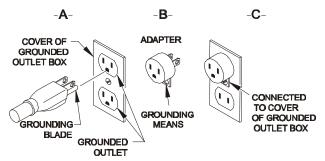
NOTE: The use of the adapter shown in Figures B and C is not permitted in Canada. If a grounding type receptacle is not available, do not use this charger until the proper outlet is installed by a qualified electrician.
