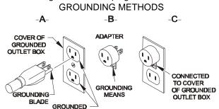
NOTE: The use of the adapter shown in Figures B and C is not permitted in Canada.
